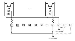
**Digital outputs.** Module Synapse has 8 Digital Outputs, which are separated in two isolated groups. There are few possible types of output circuits, such as triac (SSR) or relay (R), or their combination (4+4). Due to Zero-cross detection unit, SSR providing comfort switching any AC load in the range 85 - 220V, 2A. Relay outputs is commonly used for dry contacts and DC signals commutation.
